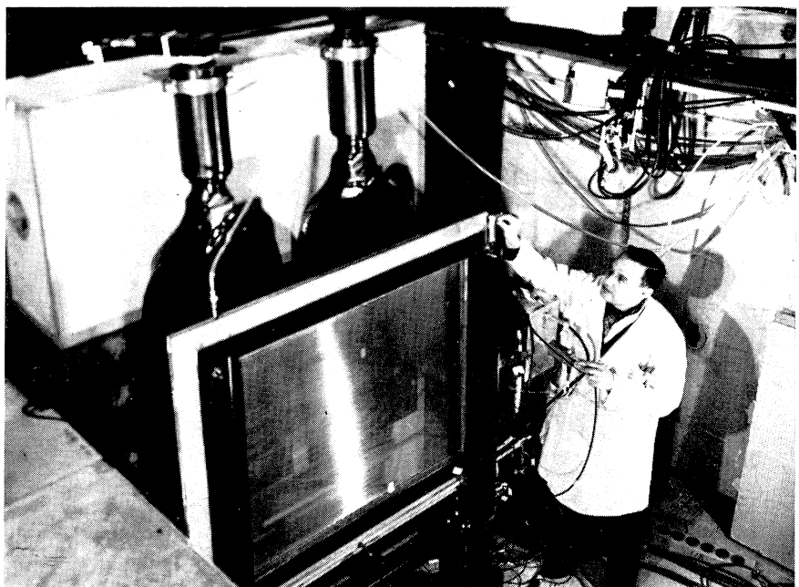
The first wire spark chamber installed in a PS experiment. Behind the chamber stand the two black shapes of scintillation counters which trigger the spark chamber when they themselves have recorded the passage of a charged particle. Behind them, below the concrete support, the block of iron (see below) is visible.
