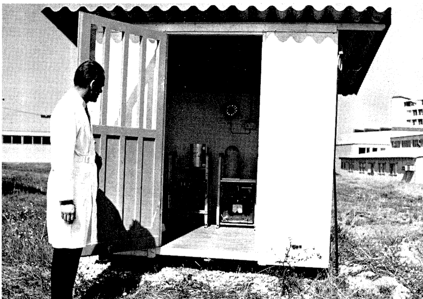
Figure 2. One of the permanent radiation monitoring stations installed on the site. It is equipped with a 'Long Counter' and an argon ionization chamber. Four of these stations have been set up on the site (the one in the photograph is close to Adams Hall) and four more are to be erected this year.
